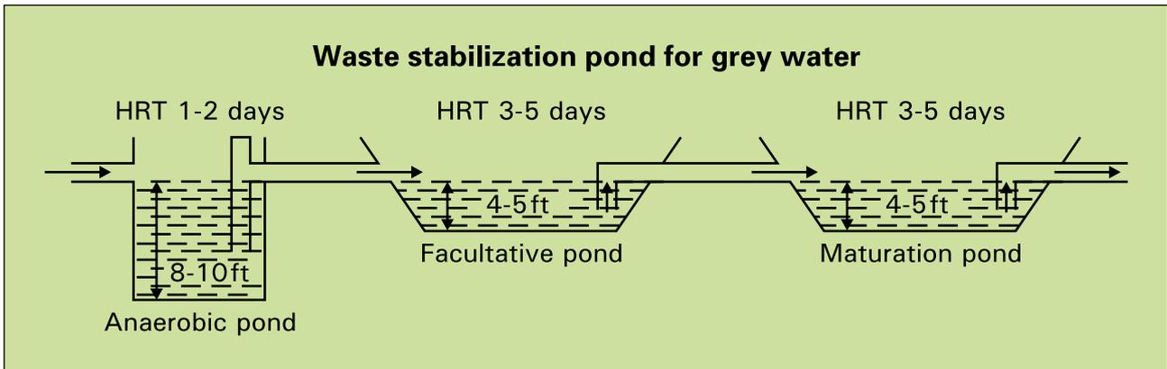
maintained while in the lower layer, anaerobic conditions exist. In this pond solids are generally taken care of by three mechanisms.
