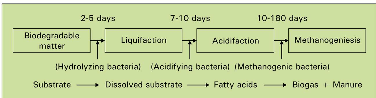
into micro-molecules with the help of some enzymes which are secreted by the bacteria. In the initial step, oxygen in the feed materials is used up by oxygen loving bacteria and large amounts of carbon-dioxide (CO<sub>2</sub>) are released and the major end product of this step is *glucose*.
