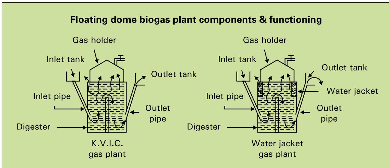
human and animal waste. It is usually built below ground level hence it is easier to insulate in a cold climate. The plant can be built from several materials, e.g. bricks, concrete, lime concrete and lime clay. This facilitates the introduction and use of local materials and manpower. The available pressure inside the plant doesn't cause any problems in the use of the gas.
